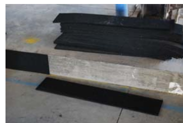
Below: FAVIM used as lateral isolation strips for floating floors.
