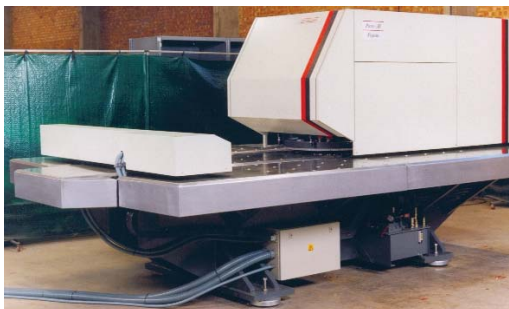
Above: Turret punch installed on Isomounts
