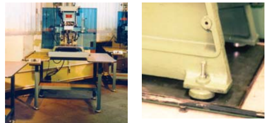
Testing Machine (Left) and Fly Press (Right), both installed on Isomounts.
