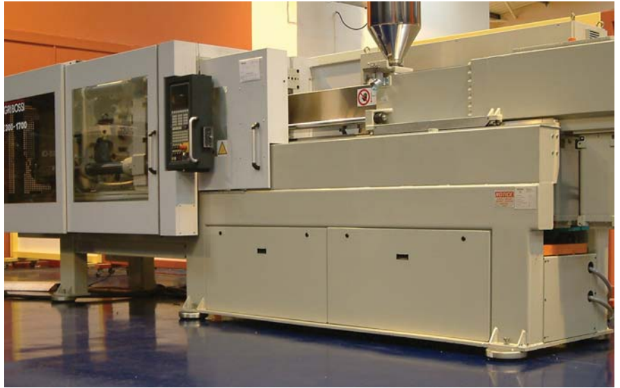
Injection Moulding machine, installed on Isomounts.
