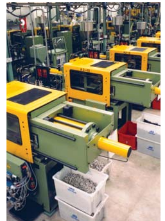
Right: Injection moulding production line installed on Isomounts
