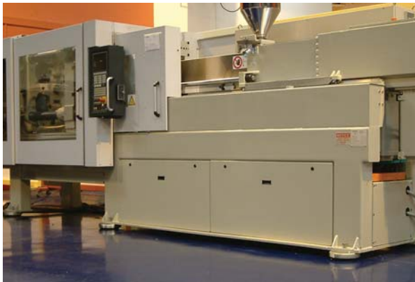
Above: Injection moulding machine installed on Isomounts
