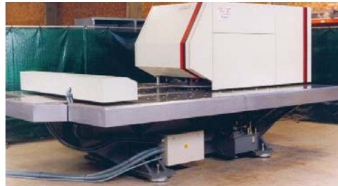
Above: Turret punch installed on Isomounts
