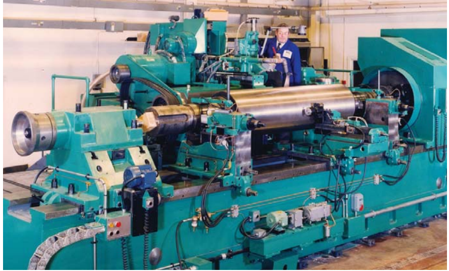
Roll grinding machine installed on Freestanding Wedge Levelling Elements (WL-LE)
