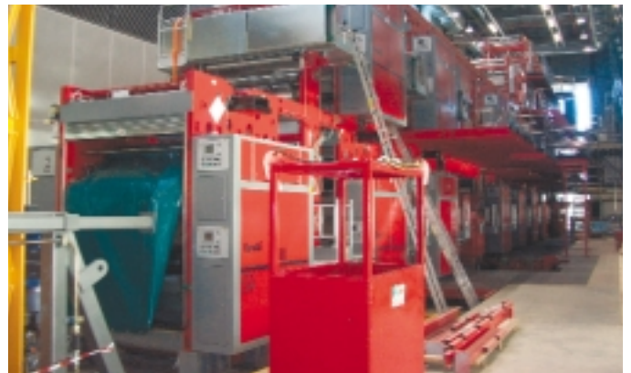
Cerutti Printing Press on ISOMAT isolated foundation
