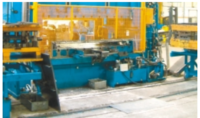
Rhodes 2500kN Power Press on ISOMAT isolated foundation
