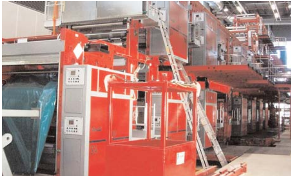
94m long newspaper printing press on Isomat Isolated Foundation.
