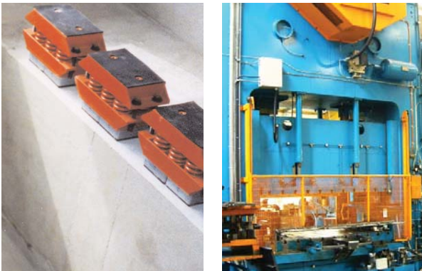
Left: Test rig on FSL coil spring isolated foundation.
