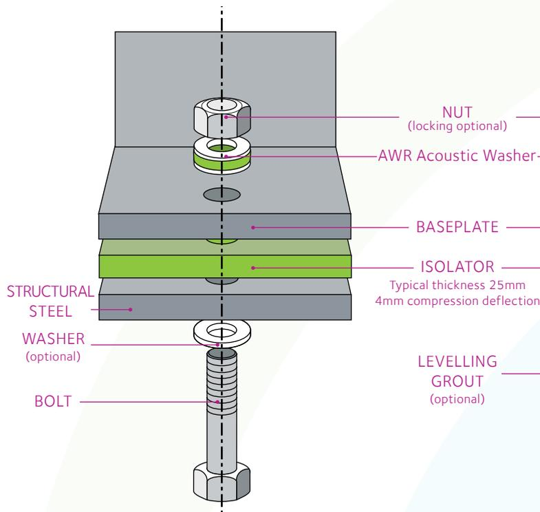
Fig 2.4 AWR - Baseplate Detail (Steel to Concrete)
