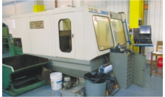
CNC machining centre on ISOLAY isolated foundation
