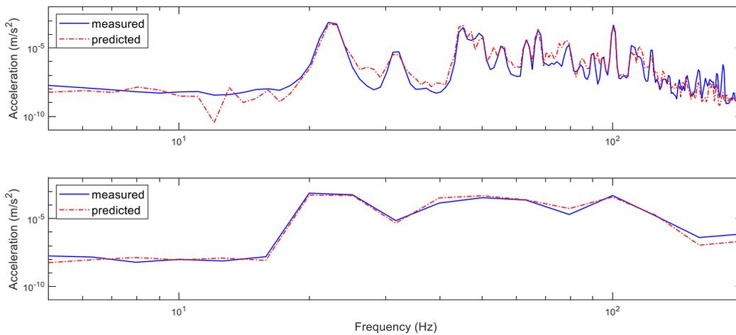
Figure 8: Logarithmic representation of the vertical acceleration measured (blue) and predicted at (e) using Eq. 8 (red-dashed) in narrow band frequency (top) and in third octave band (bottom) between 5 and 200 Hz
