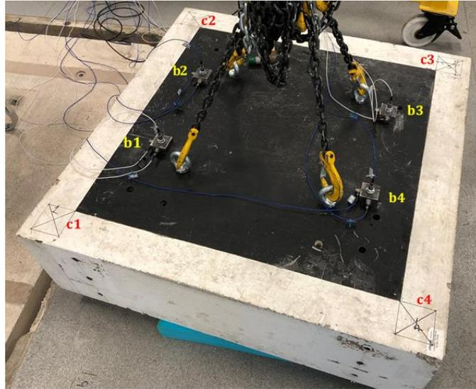
Figure 3: Inertia Block hanging, with (b) and (c) interface positions
