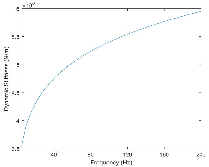
Figure 4: Dynamic compression for isolator characterisation (left) and dynamic stiffness of VM70 obtained in the vertical direction (Z) (right)
