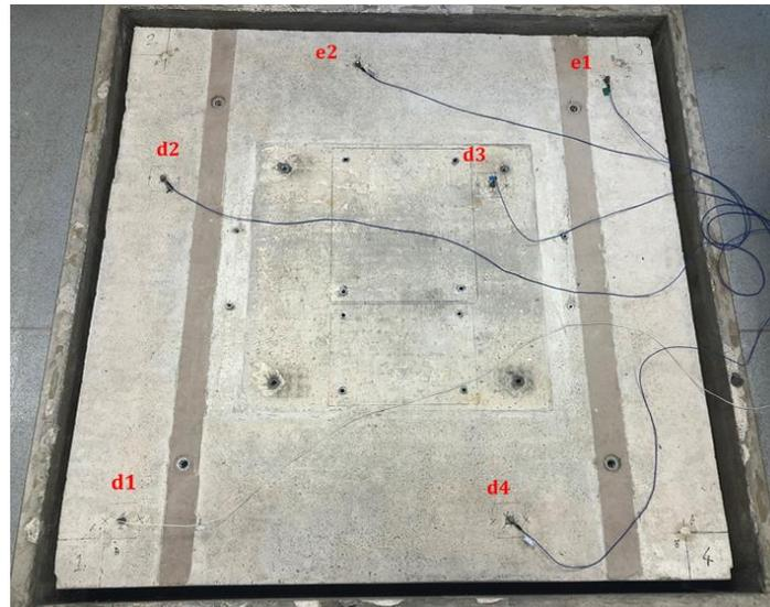
Figure 5: Receiver structure with (d) and (e) interface positions
