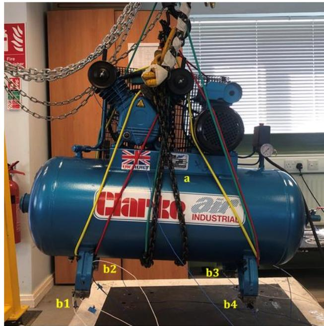
Figure 2: Vibration source hanging, with (a) and (b) interface positions
