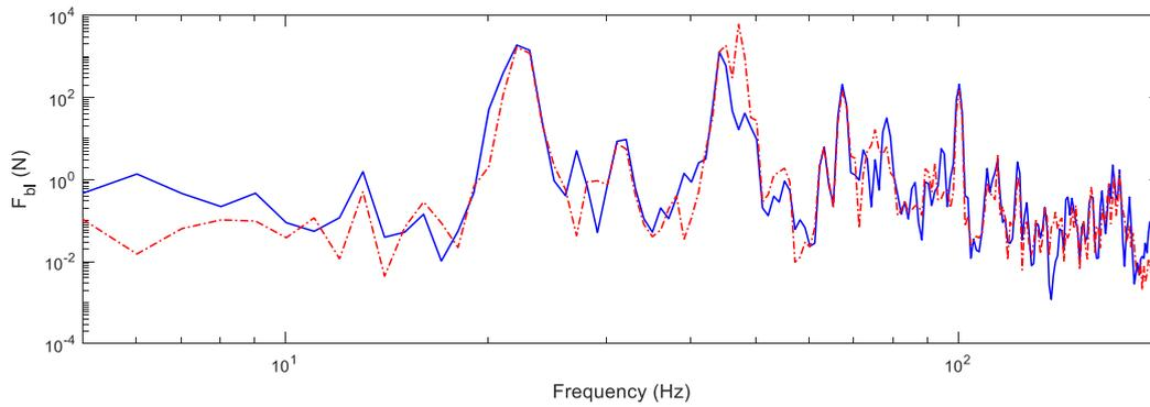
Figure 7: Logarithmic representation of the vertical blocked forces at the (c) interface using Eq. 6 (blue) and Eq. 7 (red-dashed) in narrow band frequency between 5 and 200 Hz
