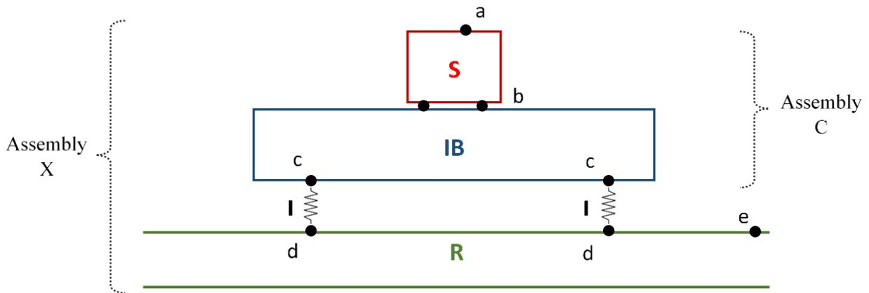
Figure 1: Assembly diagram showing the four elements (S, IB, I, R) with their interfaces (a, b, c, d, e)
