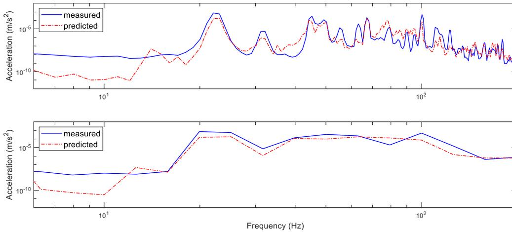
Figure 9: Logarithmic representation of the vertical acceleration measured (blue) and predicted at (e) using Eq. 9 (red-dashed) in narrow band frequency (top) and in third octave band (bottom) between 5 and 200 Hz
